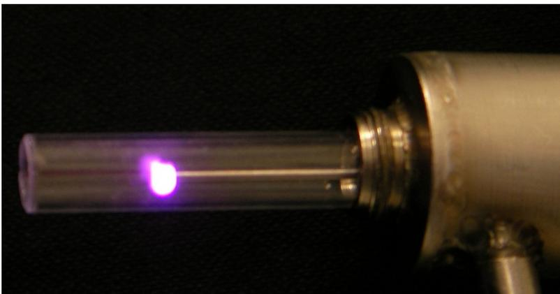
**Fig. 7: Microwave generated plasma protruding from the cylinder**
