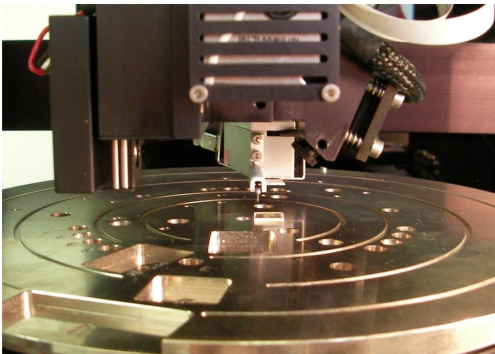
**Fig. 20:** Sample loaded on profilometer
