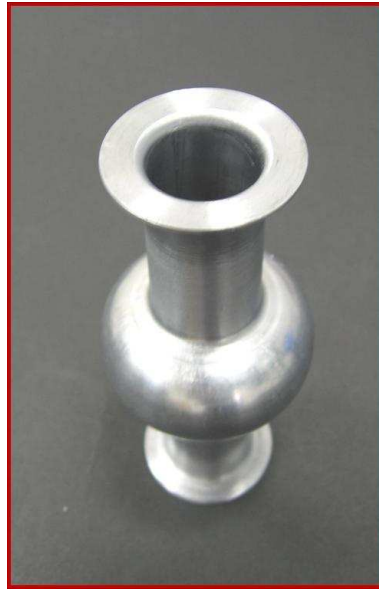
Figure 1.1: A seamless Tesla Type bulk niobium 6 GHz cavity. Spun resonators don't need welding (even for flanges).
