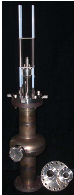
Figure 3.12: For the first attempts, the resonance atmospheric plasma has been observed (through a protective wire netting) from a glassy window fixed to the 1.5 GHz cavity cell.
