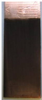
Figure 4.7: Thin brown film on copper sample after potentiostatic experiment in EMIC molten salt at -1,2V vs. quasi-Nb. (Counter electrode – niobium rod)
