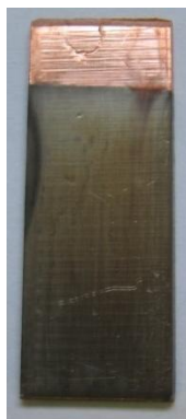
Figure 4.5: Thin gray film on copper sample after pre-electrolysis in EMIC molten salt at -0,8V vs. quasi-Nb. (Counter electrode – niobium rod)
