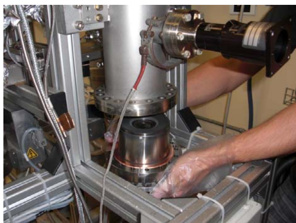
Fig. 2.18 mounting the magnetron from the bottom of the chamber
