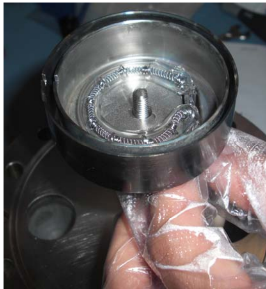
Fig. 3.6 Mounting the lamp for annealing heater
