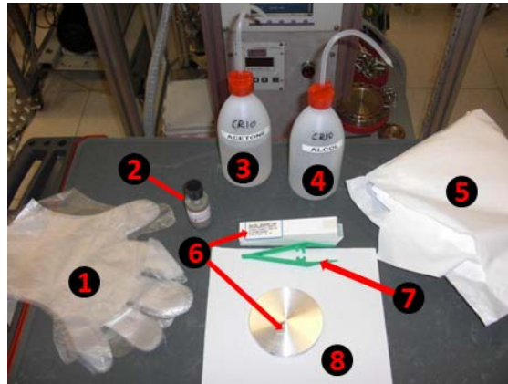
Fig. 2.21 preparation of the sapphire fixing on the holder
