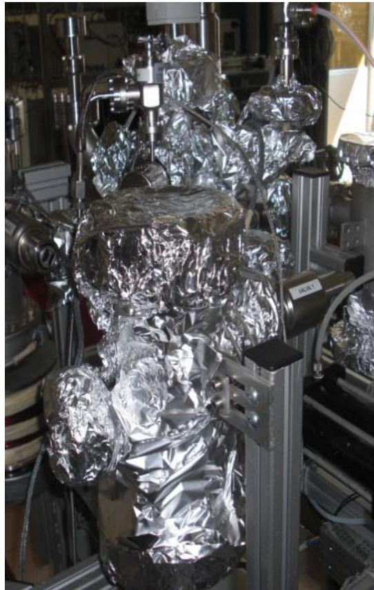
Fig. 2.14 The chamber covered with aluminum foils.
