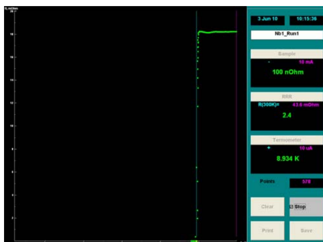
Fig. 2.32 the interface of T_c measurement less than 10K
