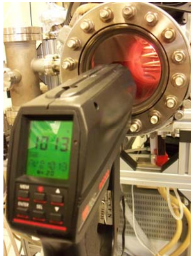
Fig. 3.31 measuring the temperature of the sample during annealing
