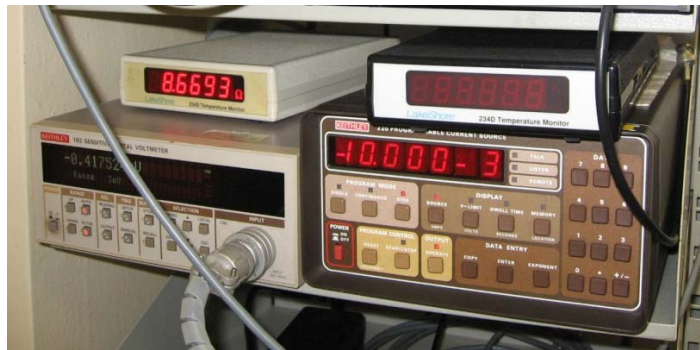
Fig. 2.28 the current source and voltage meter for T_c measurement
