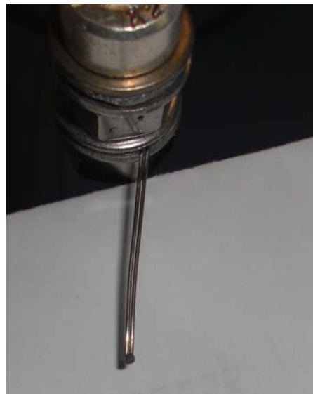
Fig. 3.8 the thermal sensor after welding
