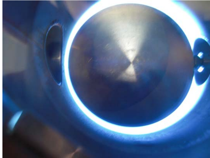
Fig. 2.23 The plasma during the sputtering
