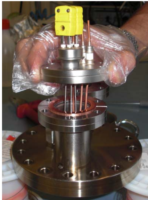
Fig. 3.10 mounting the feed through of heater and thermal sensor
