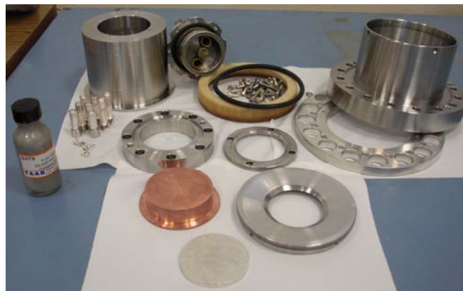
Fig.2.16 The assembly of the Nb magnetron
