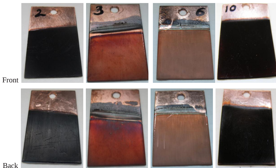
Figure.3.6. Electrochemical oxidation of copper in alkaline solution with sodium molybdate
