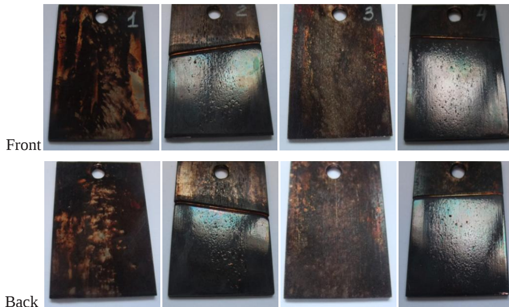
Figure.3.3. Front and back of copper samples treated in oxidation solution
