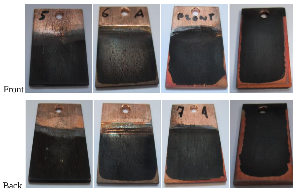
Figure.3.11. Electrochemical oxidation of copper with AC
