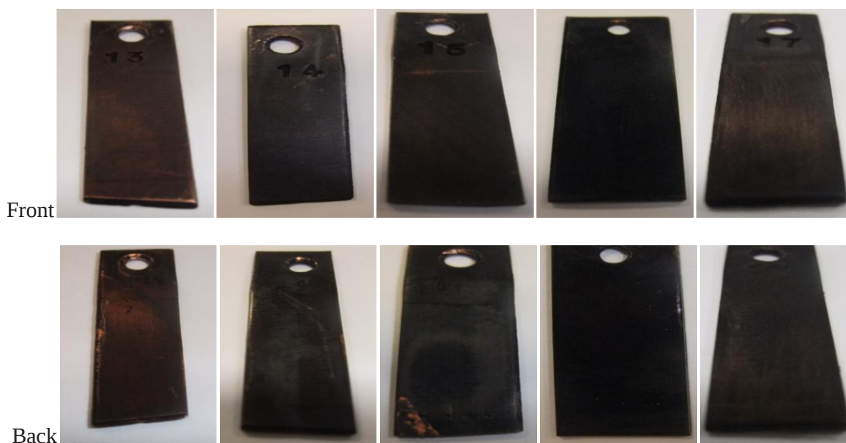
Figure.3.2. Front and back copper samples treated in oxidation solution
