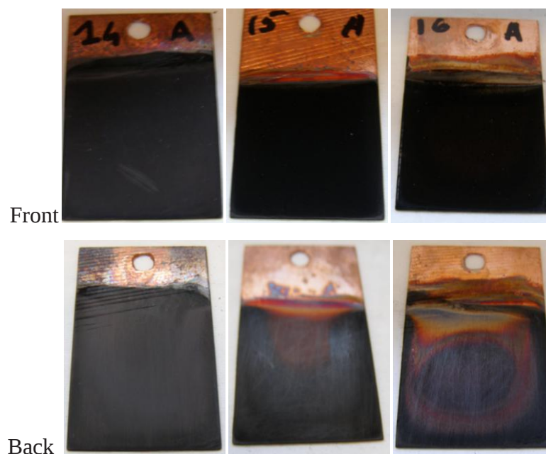
Figure.3.16. Electrochemical oxidation of copper using AC in alkaline higher concentration
