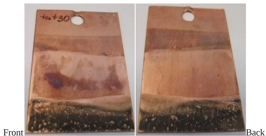
Figure.3.37. Electroplating Cr(3+) on copper substrate from ionic liquid
