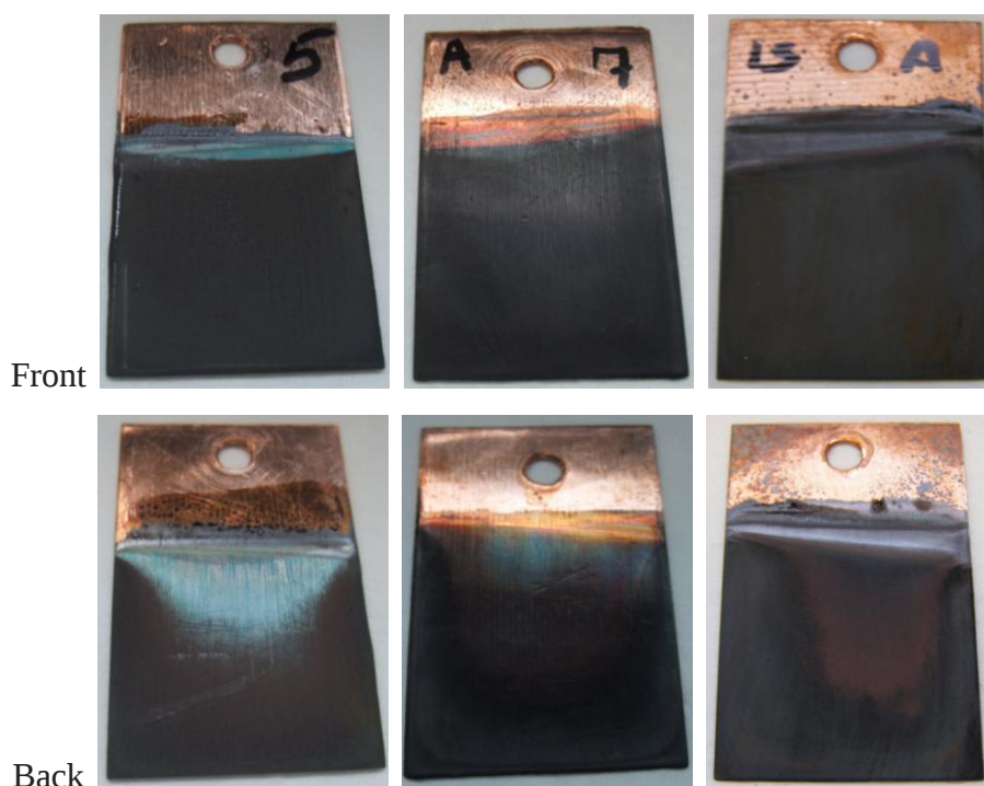
Figure.3.17. Electrochemical oxidation of cooper in different solutions
