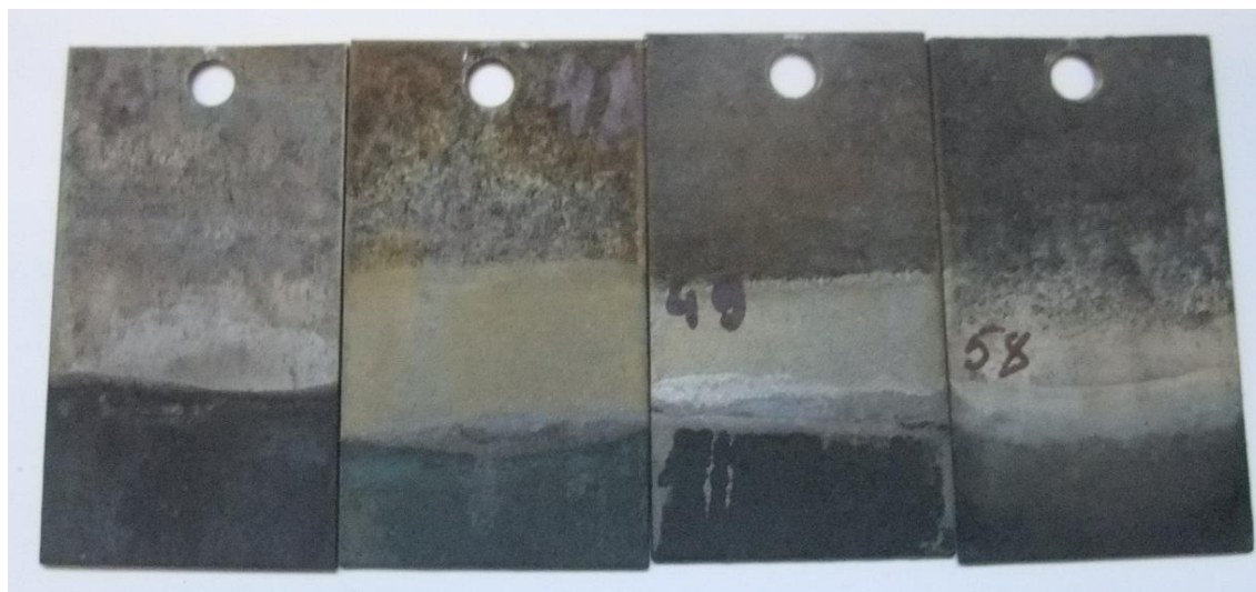
Figure3.34. Black chromium on steel substrate from ionic liquid
