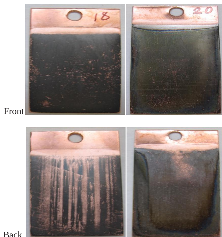
Figure.3.32. Electroplating in Pyrrole + Tiron solution
