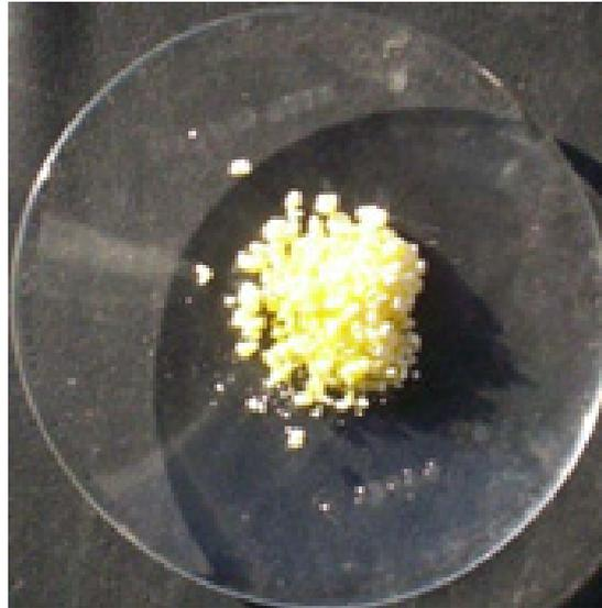
Figure 2.1: *Niobium pentachloride* ( $NbCl_5$ )
