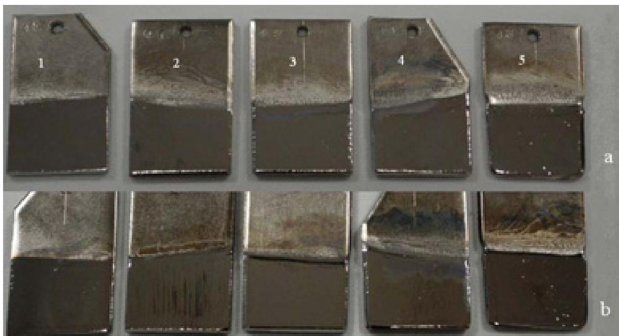
Figure 5.15: *Outward appearance of the samples electropolished with different time.*
