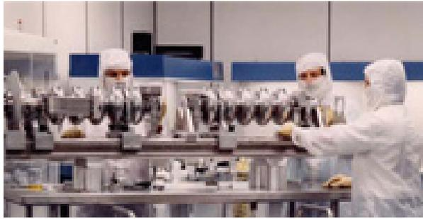
Figure 0.7: A pair of 5-cell Nb cavities developed at Cornell for CEBAF
