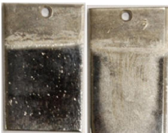
Figure 5.2: *Front(left) and back(right) of sample electropolished with overpotential 30 V.*
