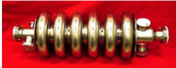
Figure 0.8:  $b = 0.6$ , 6-cell cavity for SNS, frequency 804 MHz
