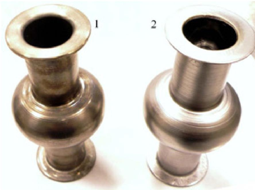
Figure 3.5: *Difference between flanges surface before(1) and after(2) lapping.*
