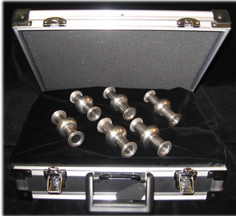
Figure 3.4. 6 GHz Nb cavities, produced by spinning technology
