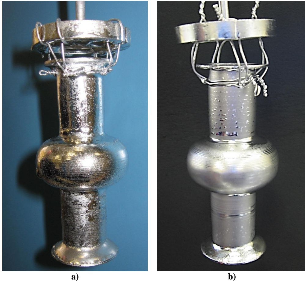
Figure 7.12. Cavity after dipping step. Cavity №5 (a) produced without post heating, and cavity № 25 (b) produced with post heating
