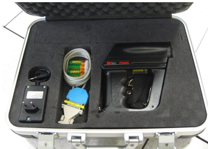
Figure 7.6. Pyrometer IRtec P-2000
