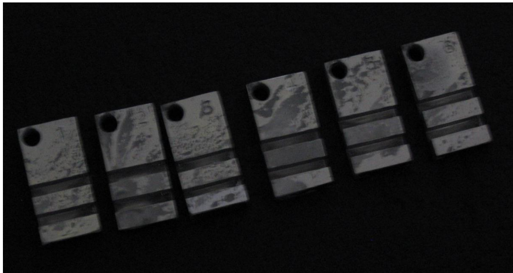
Figure 7.8. The photograph of LL-samples 1-3, 2-3, 3-3, 4-3, 5-3, 6-3 after annealing in the induction oven
