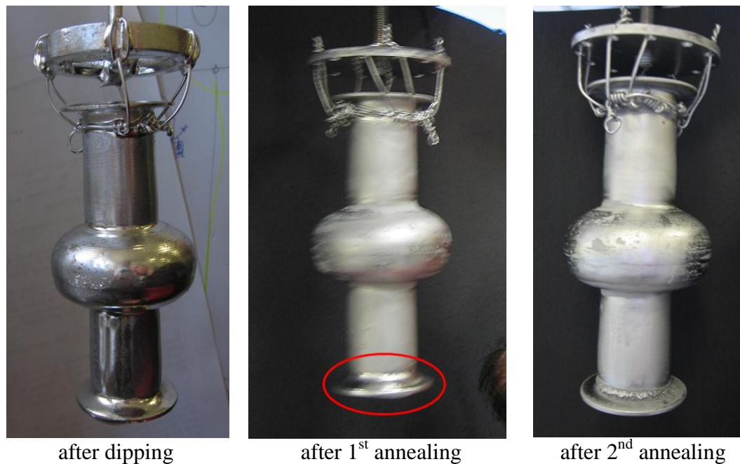
Figure 7.16. Results of annealing cavity №33
