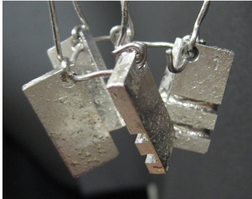
Figure 7.2. Film obtained as the result of dipping on LL – samples
