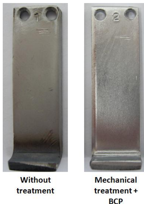
Figure 6.1. L-samples with and without BCP
