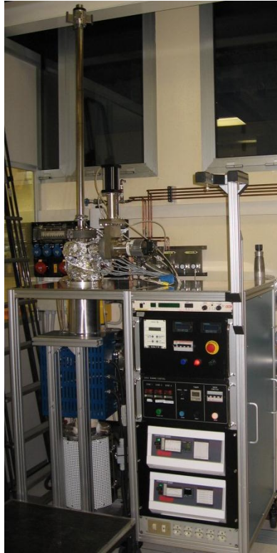
Figure 6.10. Photograph of the liquid tin diffusion experimental stand
