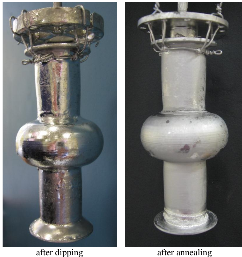
Figure 7.18. Results of annealing cavity №5
