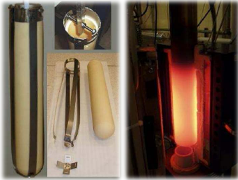
Figure 2-18 On the left the Al 2 O 3 vessel containing Sn can be extracted with a long metallic rod which can be hooked up to the inconel jacket that encloses the crucible. On the right the lower part of the system can be heated by an irradiating furnace
