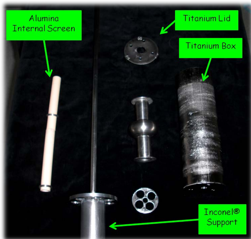
Figure 2-12 All the parts that compose the stand that enter into the furnace.
