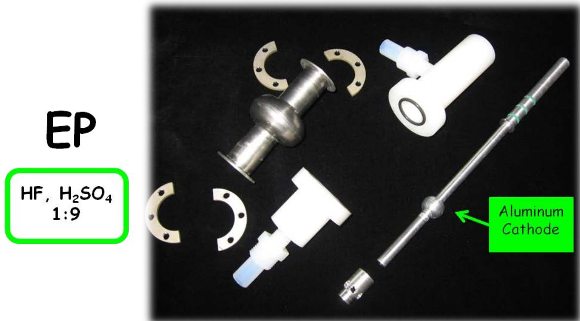
Figure 2-10 Details of the cavity closing system for electro polishing. The aluminum cathode, that enters inside the cavity, is shaped to maintain constant the cathode – internal surface cavity distance.
