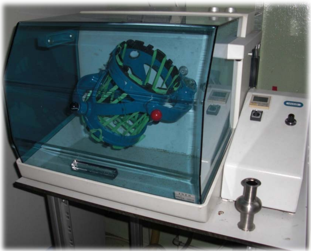
Figure 2-5 Compact tumbling system for small resonators.
