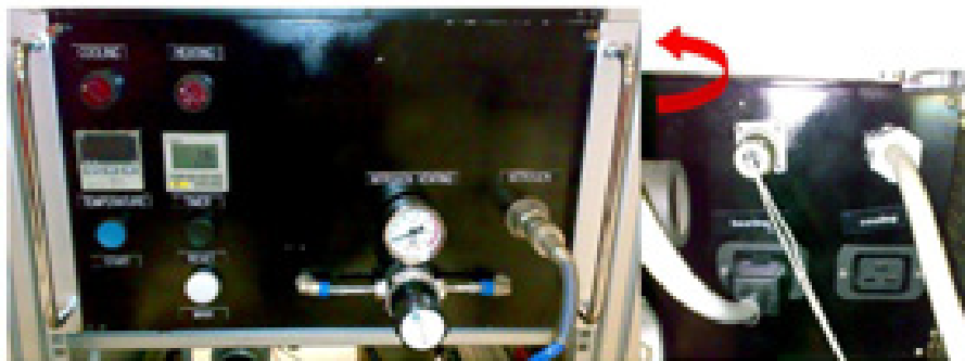
Figure 4.12: Multifunction box: from the front panel the operator can set an additional baking units and he can also regulate the nitrogen gas pressure. In the rear panel there are two sockets for the heating collar or the cooling fan plugs. One thermocouple is connected to the heating unit.
