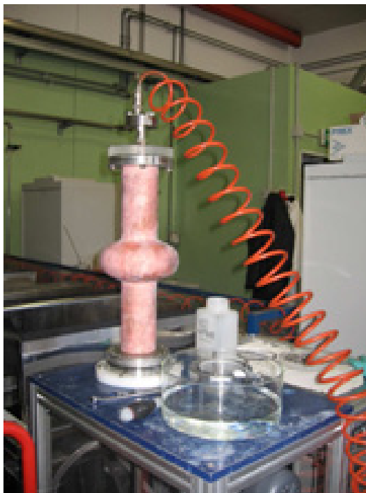
Figure 3.4: Picture of the copper cavity mounted on the HPWR system.
