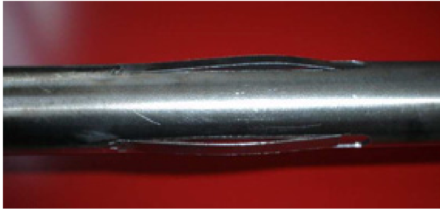
Figure 4.5: Detail of the steel tabs built up to guarantee a good electric contact between the stainless steel tube and the Niobium target.
