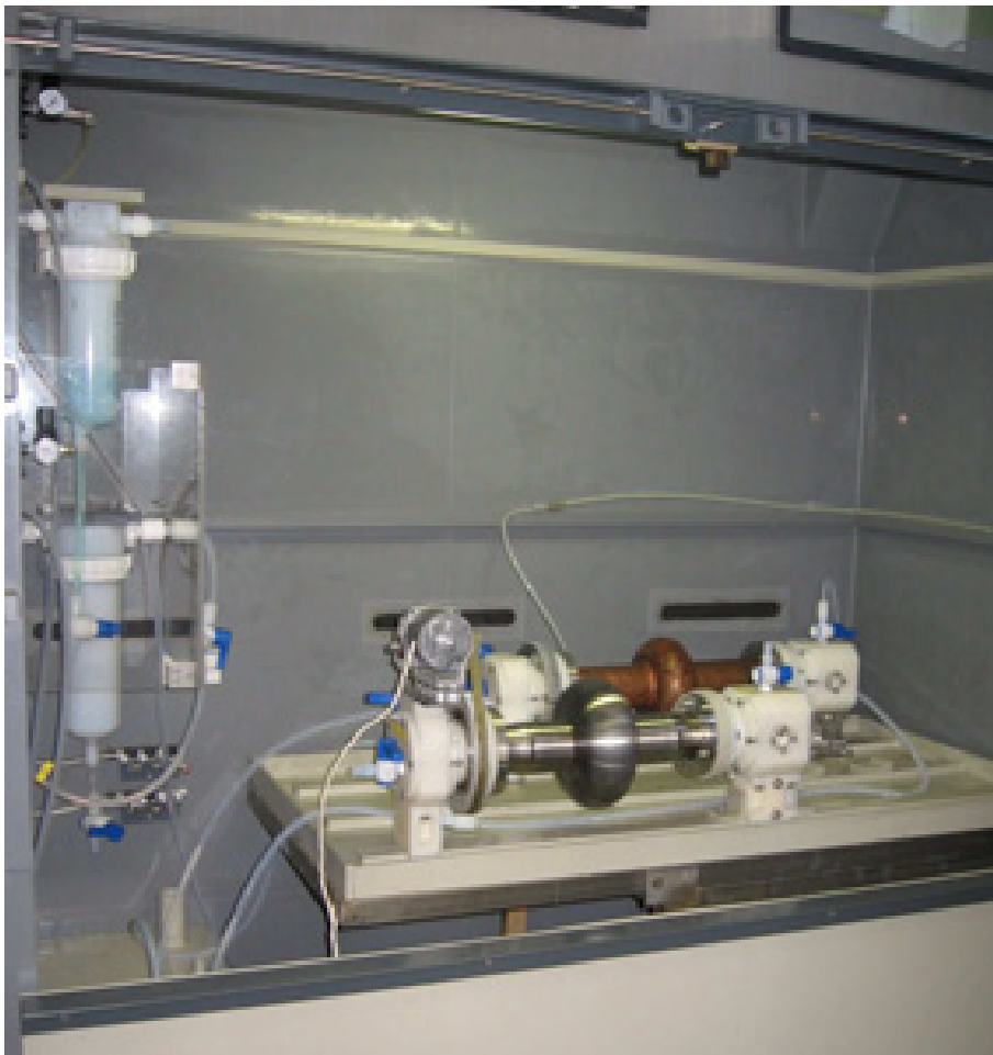
Figure 2.2: The double horizontal EP apparatus for copper and niobium cavities
