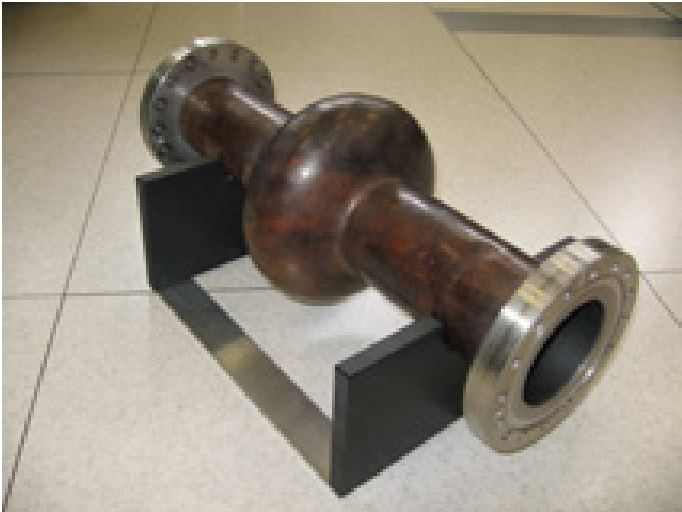
Figure 4.10: The copper cavity on its seat.
