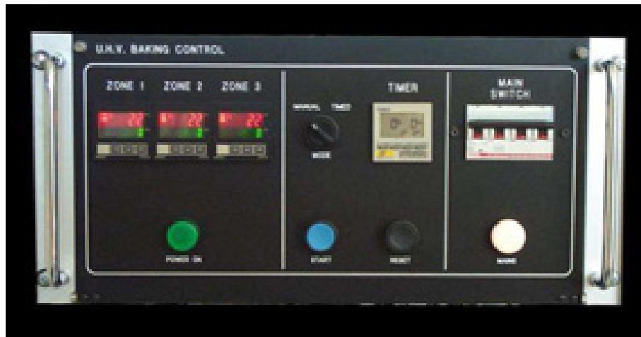
Figure 4.11: Front panel of the "UHV BAKING CONTROL" heating box.
