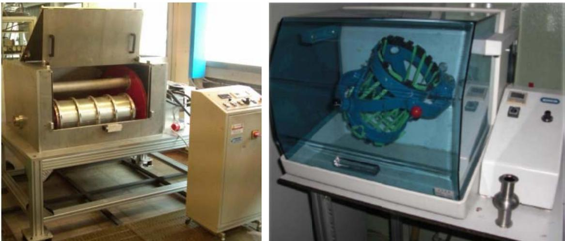
**Figure 3.2:** Left fig: Centrifugal tumbling system for multiple 6 GHz cavities. One can tumble 6 cavities at a time. Right fig: A compact tumbling system for a single cavity, cavity is tumbled in zig-zag motion.
