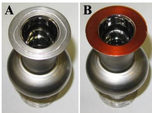
**Figure 5.5:** Fig.A: classical Indium gasket above cavity flange. Fig.B: a new Kapton Gasket
