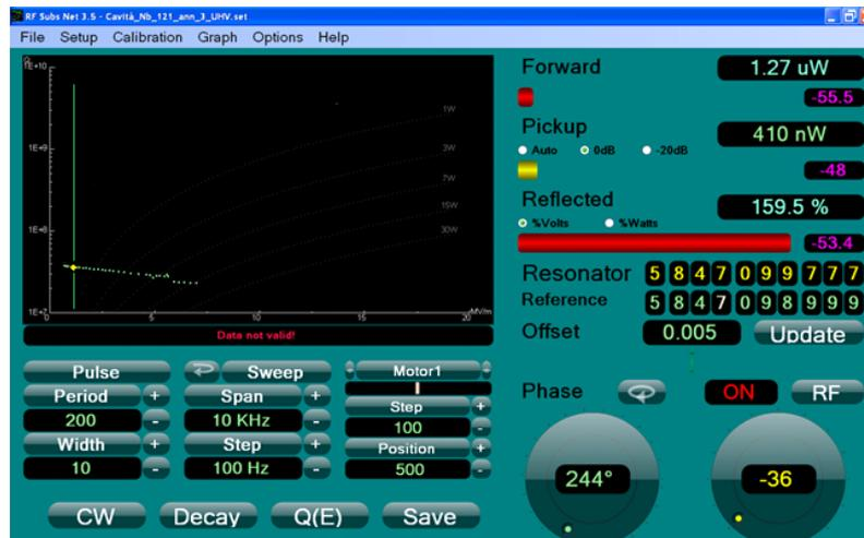
**Figure 5.17:** Measured data points are shown at 4.2K. Such data points are measured by increasing power then reducing reflected power below 5%.
