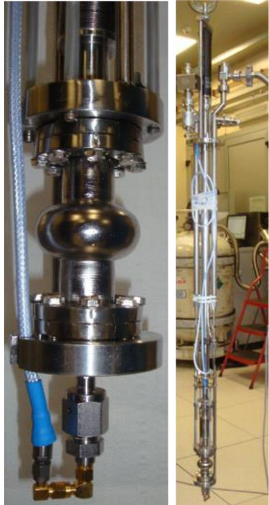
**Figure 5.4:** Cavity screwed on forward power flange (top), and pick up flange (bottom). RHS figure: Cavity pumping lines are connected to RF stand (A complete RF insert)
