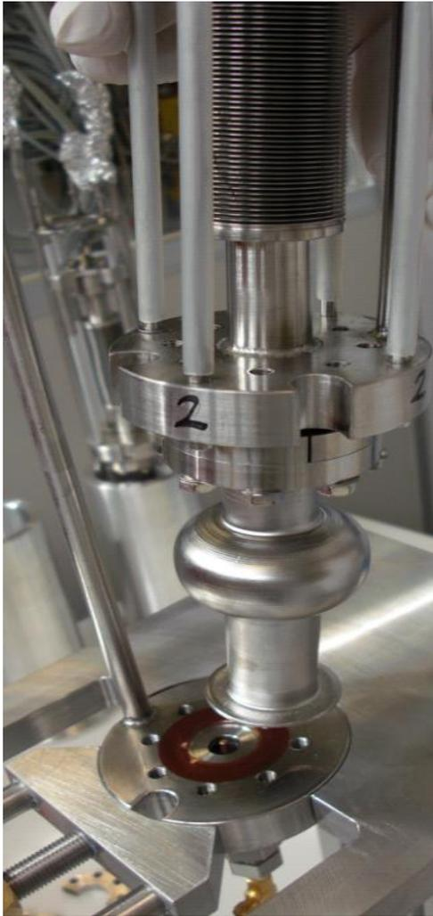
**Figure 5.3:** Cavity mounting procedure on RF stand inside clean-room
