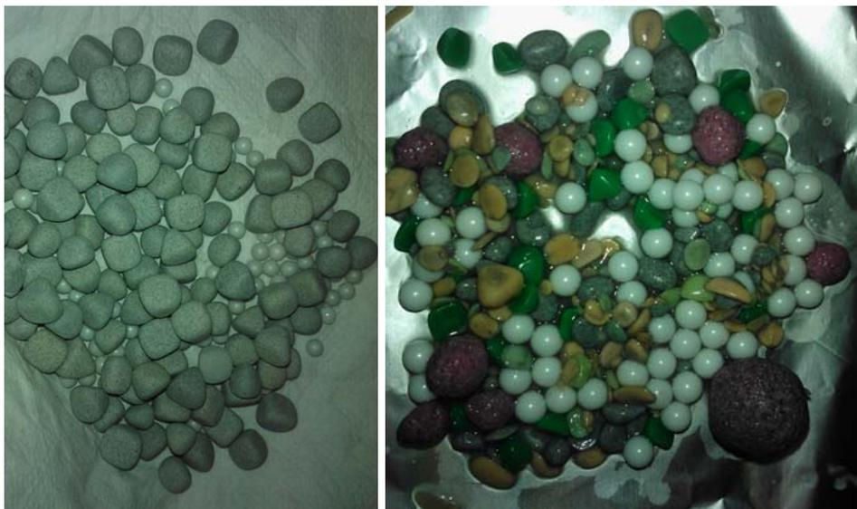
**Figure 3.5:** An abrasive agent pieces reduced in small size after 4 hours of tumbling process. **Left fig:** Silicon Carbide (SiC) and Yttria stabilized Zirconium oxide (ZrO<sub>2</sub>-Y) balls. **Right fig:** after final finishing residuals of media; SiC, ZrO<sub>2</sub>-Y, Al<sub>2</sub>O<sub>3</sub>+SiO<sub>2</sub>
