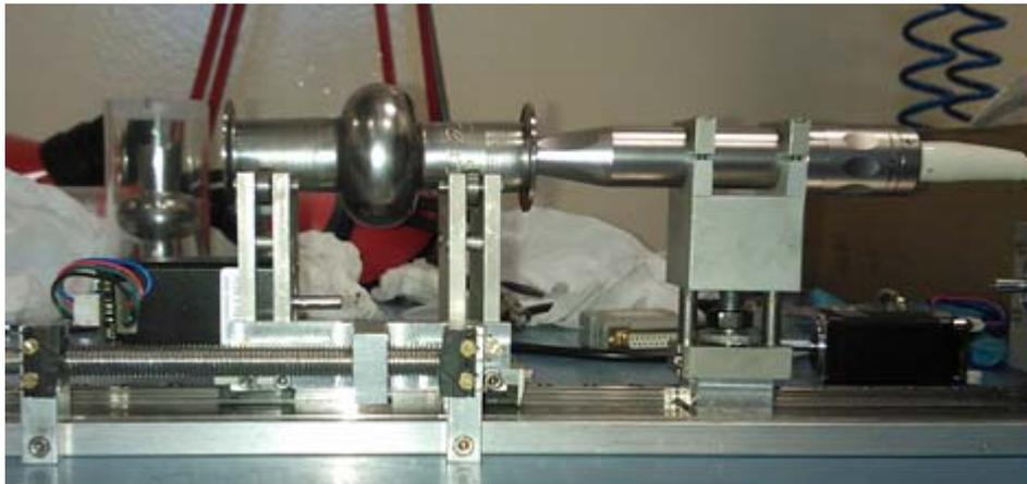
**Figure3.8:** An optical inspection set up for Inner surface of cavities is shown.
