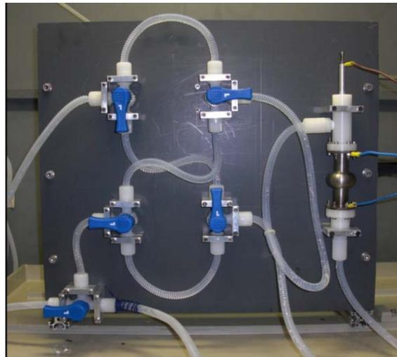
**Figure3.10:** Chemical and electro-chemical layout for BCP and EP process at INFN/LNL
