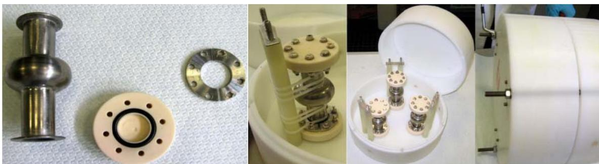
**Figure 3.3:** Left fig: 6 GHz cavity, plastic flange with viton O-ring is shown. In next figures: Cavity enclosed with abrasive media fastened at post inside the box, 3 cavities fastened in a box, and closed box (extreme right fig), which in turn placed inside metal box of centrifugal tumbling system is shown respectively. Two box, each contains 3 cavities can be tumbled at a time.
