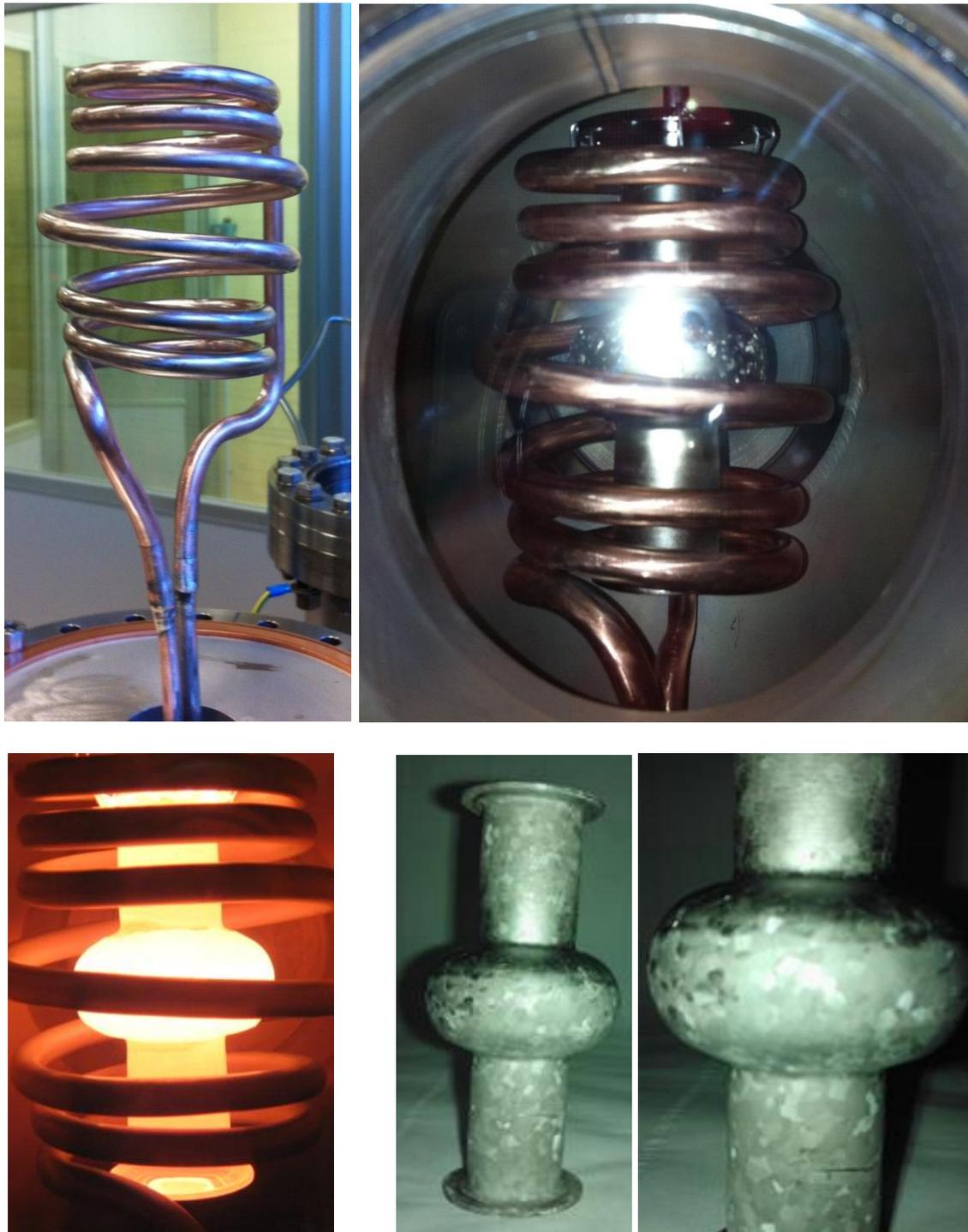
**Figure 4.9:** Induction coil designed for heating 6 GHz tesla type cavities (top-left fig.); Nb cavity inside induction coil in UHV chamber (top-right fig.); Nb cavity during high temperature annealing inside UHV chamber (bottom-left fig.); Nb cavity after high temperature annealing (bottom-middle and right figures.)
