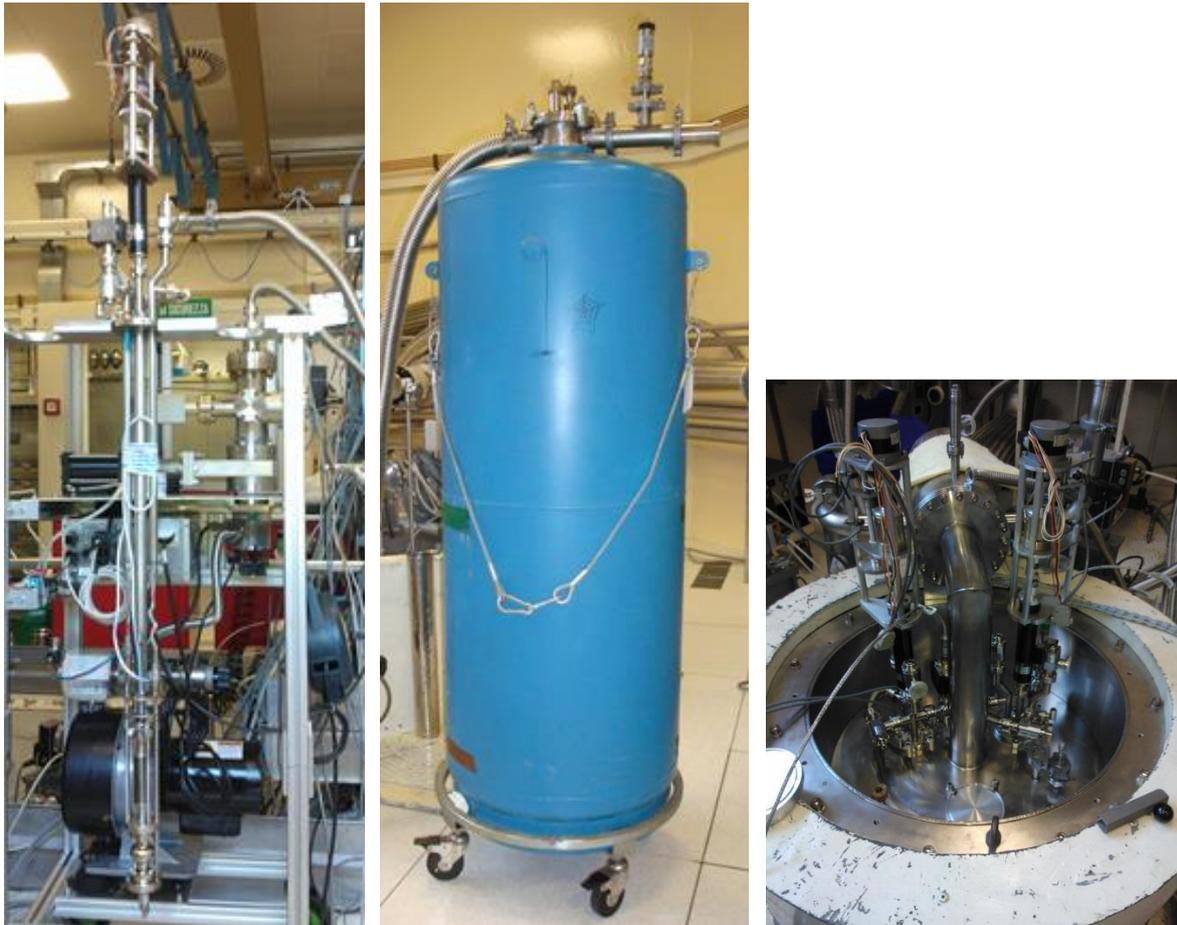
**Figure 5.2:** **Left Fig.:** A picture of 6 GHz rf cavity mounted on test stand (before being lowered into the Cryostat) with pumping system for 4.2/1.8K test. **Middle Fig:** Cryostat (Blue) for single cavity test. **Right Fig** is the cryostat for triple cavity rf test inside clean-room is shown.
