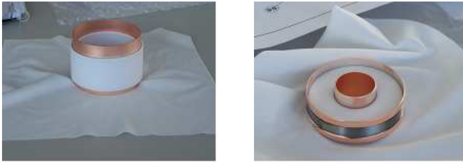
Figure I-5: TTF-III brazed cylindrical alumina coupler window (A), TW60 brazed disk alumina coupler window (B).
