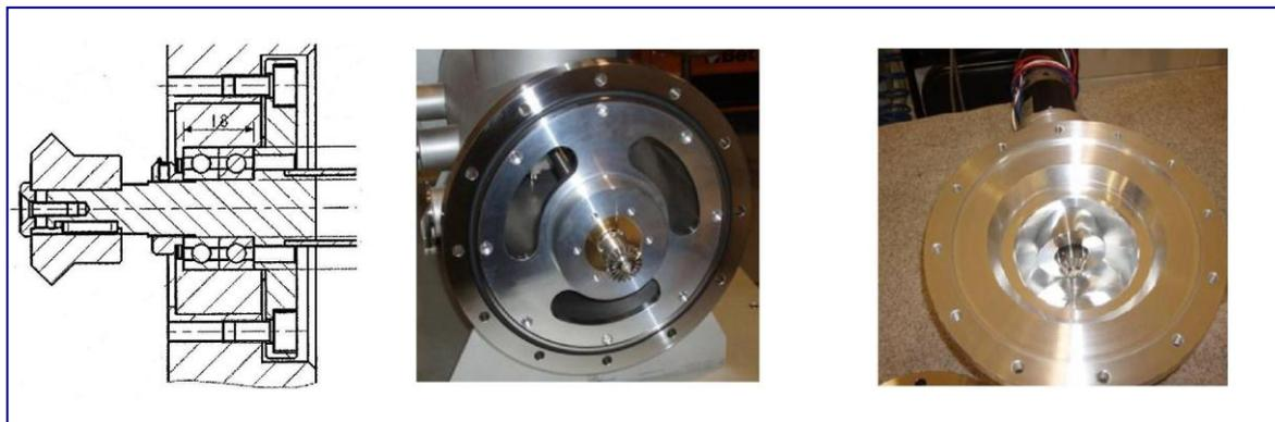
**Figure 5.18. - Detail of W6002RT4K4296 bearing. LEFT: mechanical drawing. CENTER: photography of the shaft ending with the conic gear corresponding to the mechanical drawing. RIGHT: photography of the conic gear connected to the electrical motor.**
