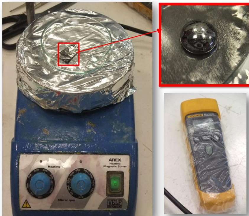
Fig.2. 14 Experimental set-up for static liquid gallium test
