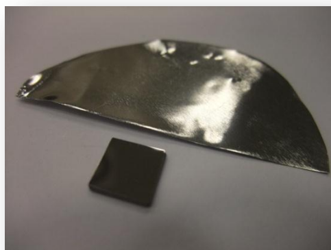
Fig.4. 2 Obtained niobium coating at 22 °C substrate temperature
