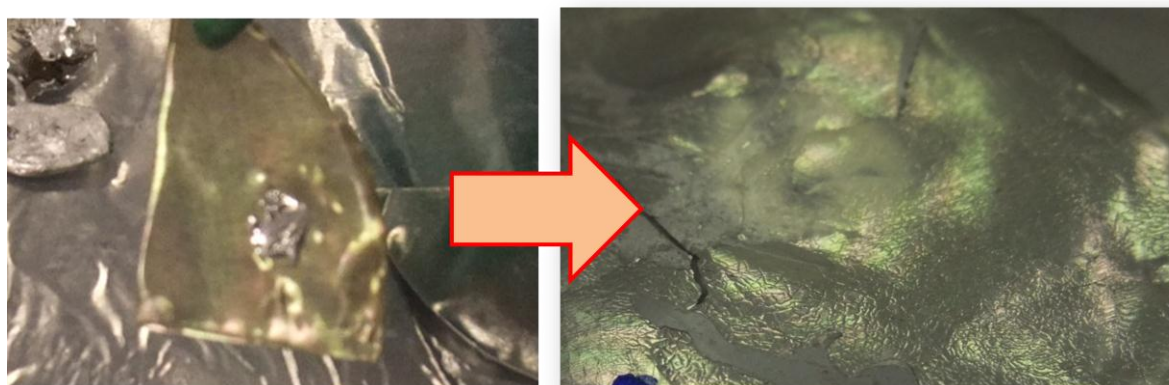
Fig.6. 10 Penetration of Ga into CeO 2 coating obtained at room temperature
