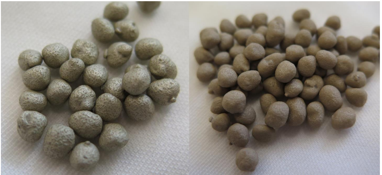
Figure 4.13: CD-13. (a) After deposition. (b) After tumbling post sputtering.
