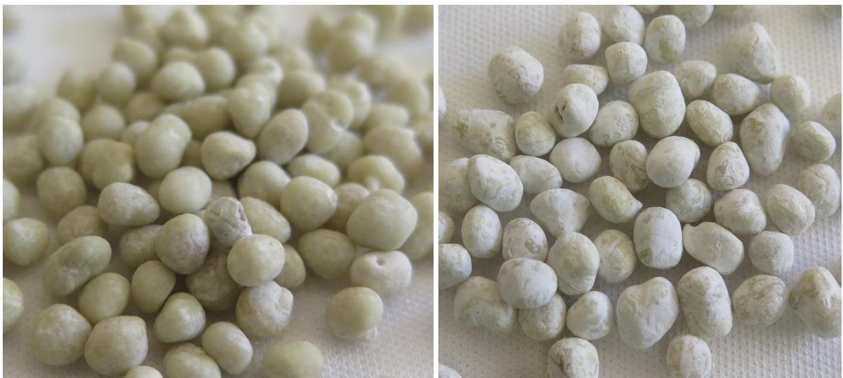
Figure 4.14: CD-14 A (5 minutes dissolution) and B (seven minutes dissolution) before coating.
