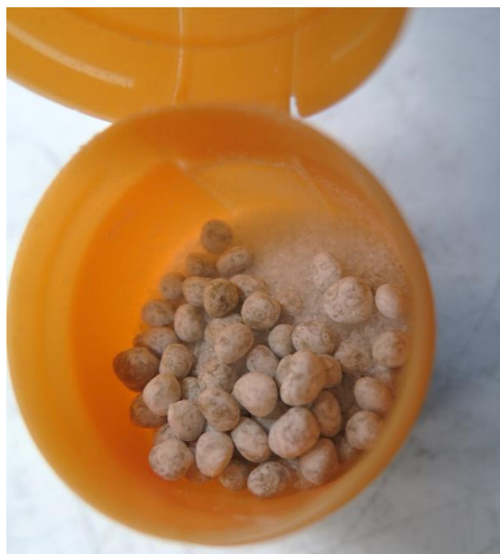
Figure 4.1: Prepared seeds to be put in the tumbler machine before deposition.
