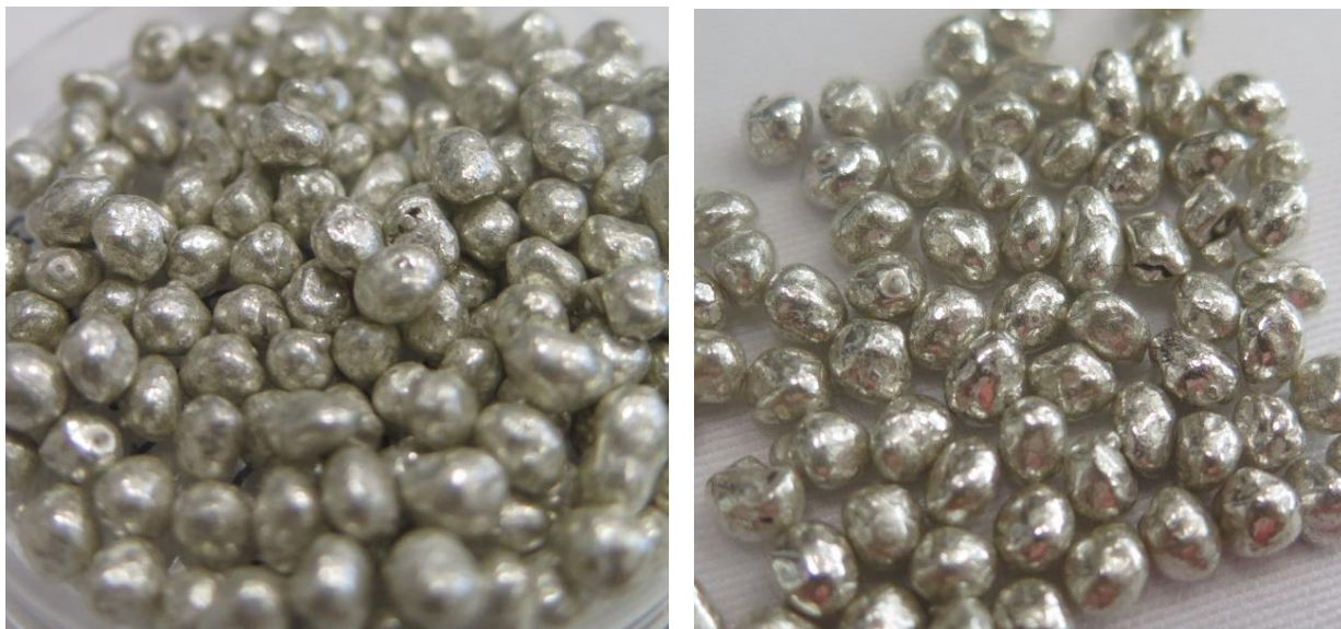
Figure 4.12: Comparison between CD-12 seeds before and after post sputtering treatment.
