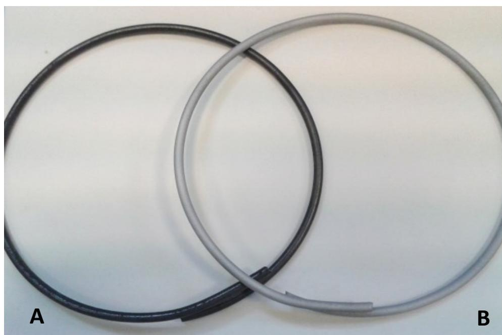
*Figure 8.4: The wire rod A - before and B - after the pulse reverse finishing in solution "C".*
