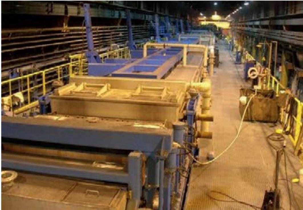
*Figure 1.6: Mixed-acid etching line. [8]*
