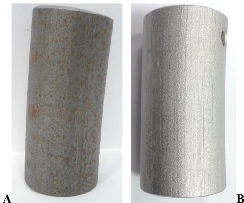
*Figure 9.2: The stainless steel sample A- before and B- after electrochemical polishing*
