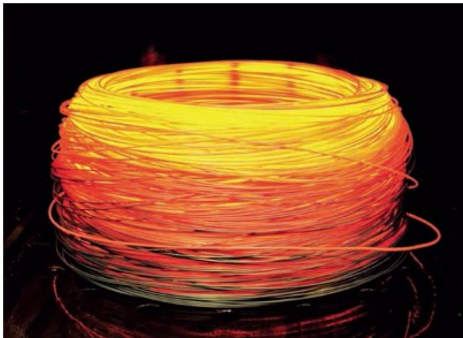
*Figure 1.5: The hot rolled rod coil.*
