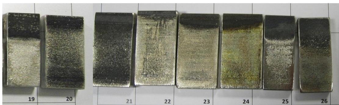
*Figure 5.13: Samples after electropolishing, back from 19 to 26.*
