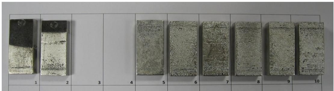
*Figure 5.4: Samples after electropolishing, front from 1 to 10.*
