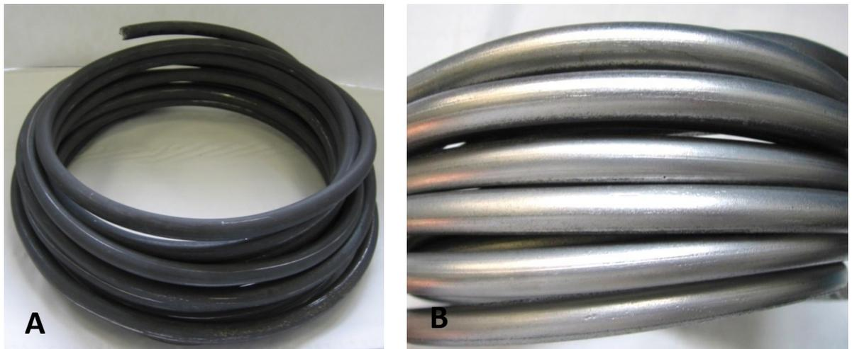
Figure 6.6: The rod with overlapped coils A- before and B- after electropolishing.
