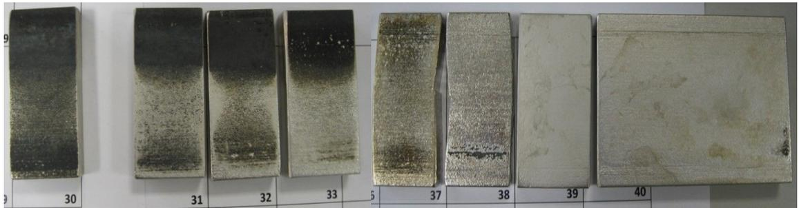
*Figure 5.16: Samples after electropolishing, back 30-40.*
