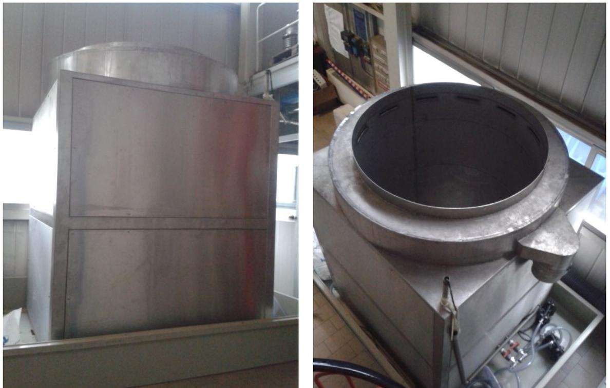
*Figure 9.3: The working bath, made of stainless steel.*
