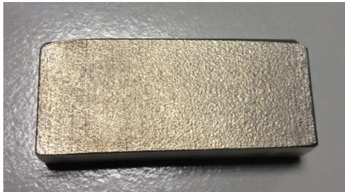
*Figure 5.23: Sample of the sulphur doped steel after electropolishing.*
