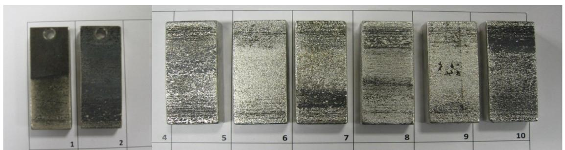
*Figure 5.5: Samples after electropolishing, back from 1 to 10.*
