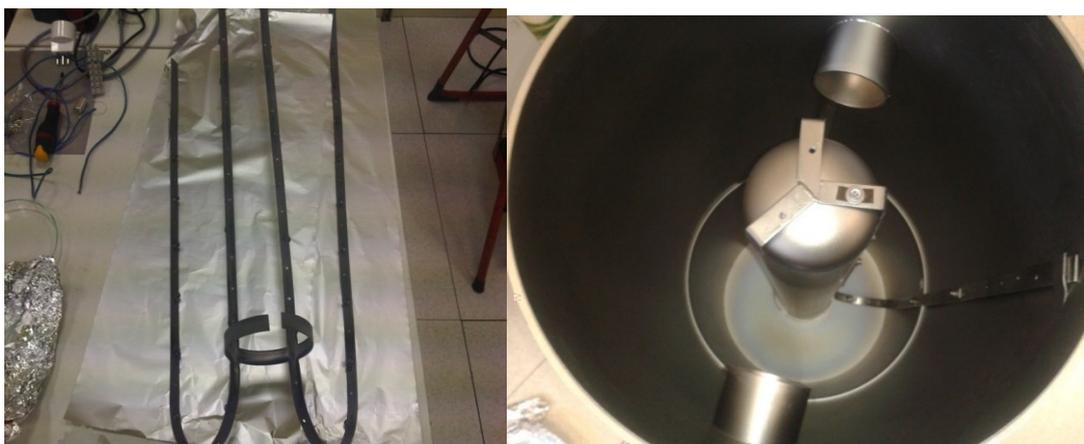
Figure 6.4. a) Sample holder b) sample holder on the QWR cavity.
