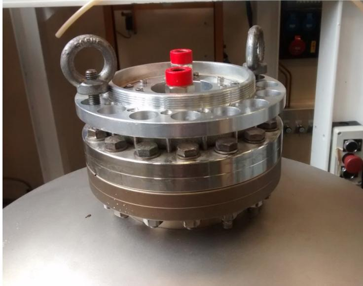
**Figure 6.9. Niobium magnetron placed on the top of the vacuum chamber.**
