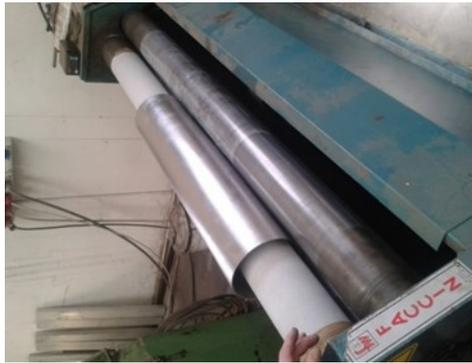
**Figure 5.4. Procedure used in the construction of the Nb.**
