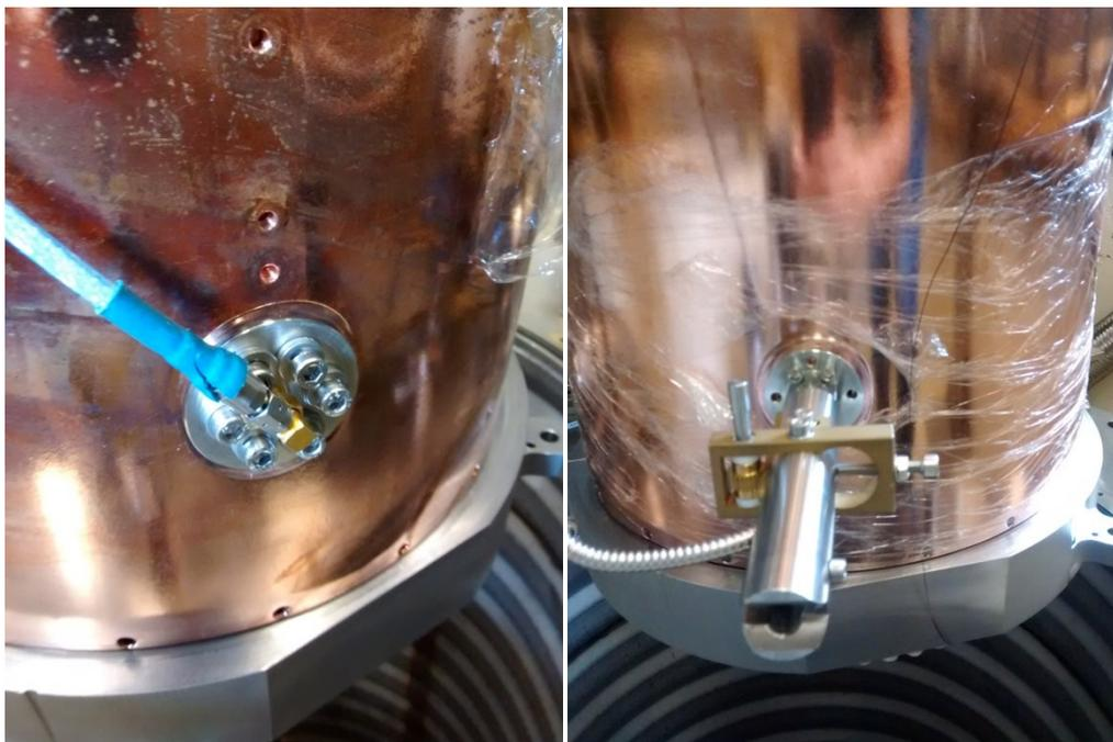
**Figure 7.9. On the left side the pick-up antenna and on the right side the coupler antenna, both during the mounting.**
