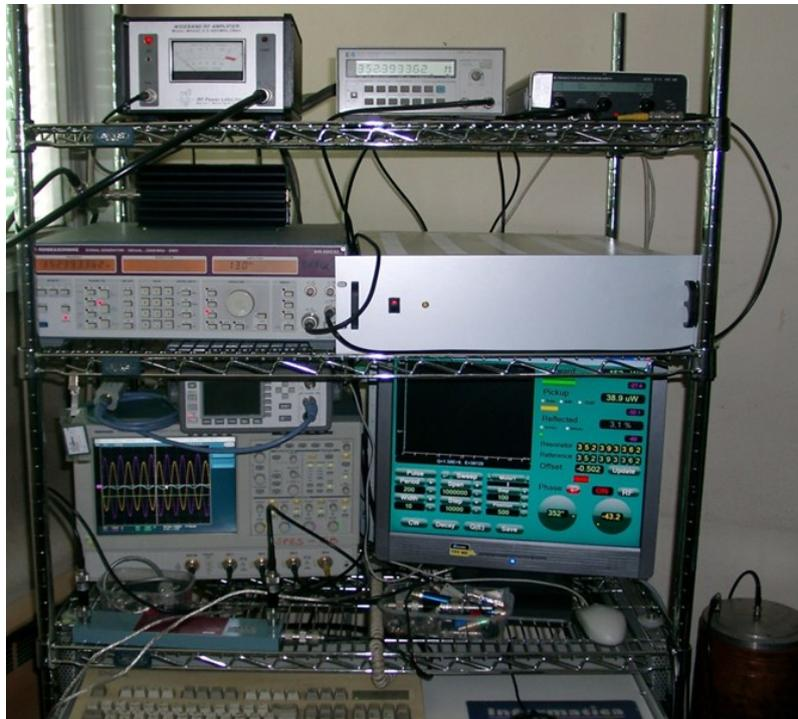
**Figure 7.7. Measurement system for cavity testing [61].**
