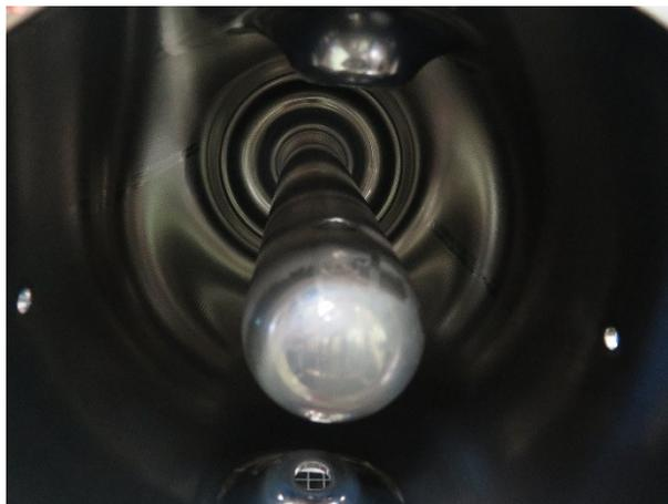
**Figure 8.38. Nb/Cu QWR cavity after the high pressure rinsing.**
