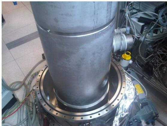
Figure 6.6. QWR during the mounting on the vacuum chamber.
