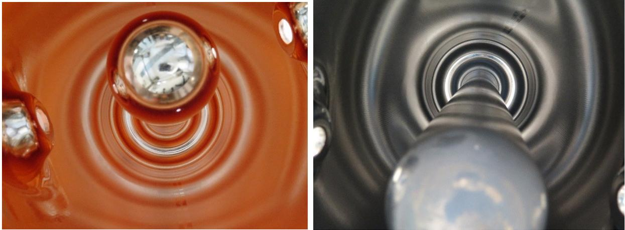
**Figure 8.37. QWR cavity before and after the Nb deposition.**
