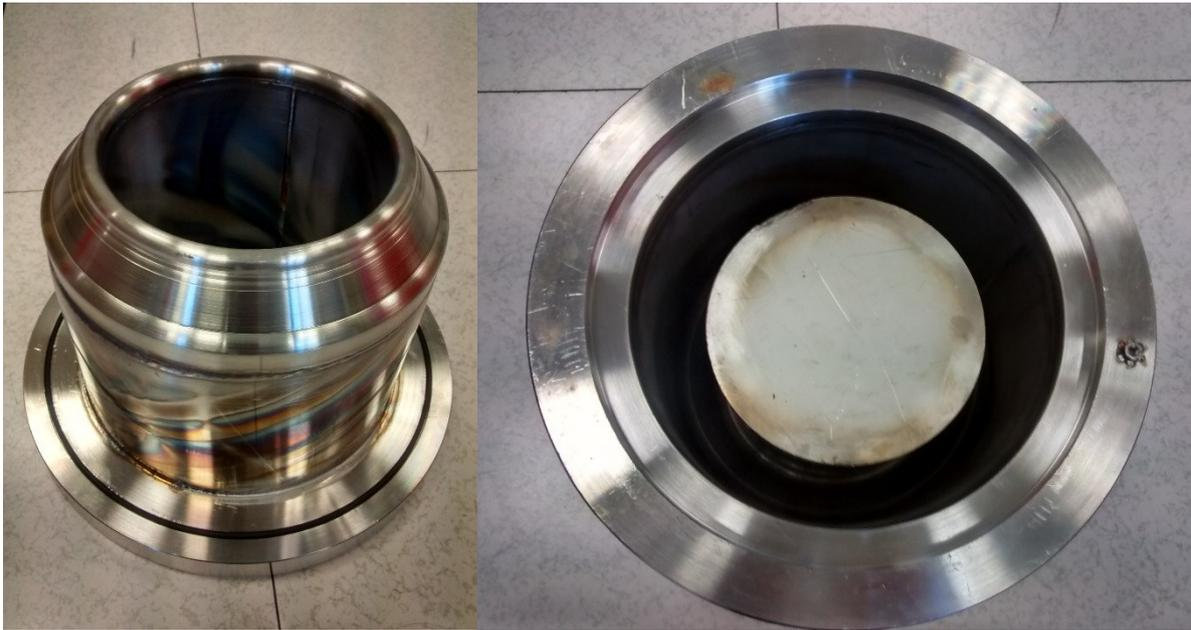
**Figure 6.1 a) Stainless steel test cathode, b) top view of the test cathode.**
