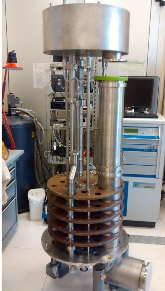
**Figure 7.2** Upside down of the cavity stand during the cryostat mounting.
