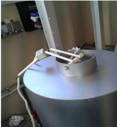
**Figure 8.18. IR lamp placed inside the central electrode of the QWR**
