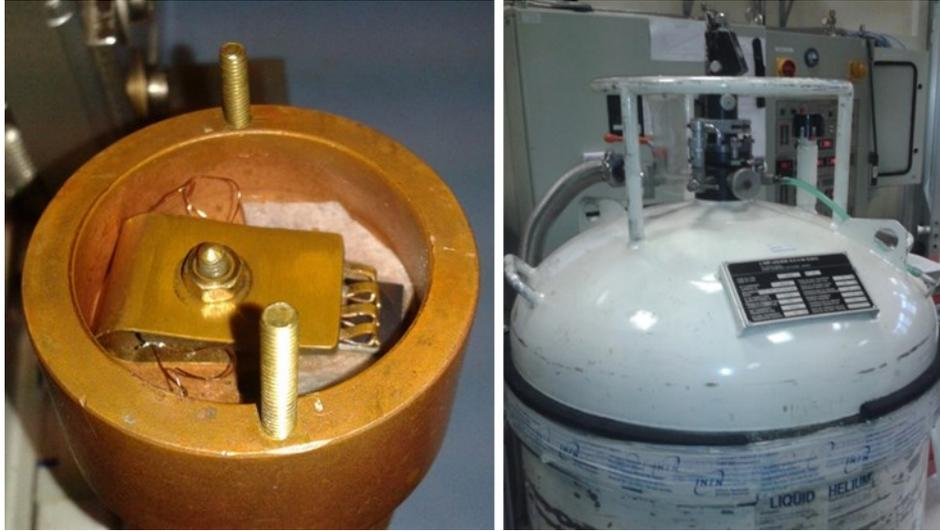
**Figure 6.14. a) Resistive sample holder. B) Helium Dewar.**
