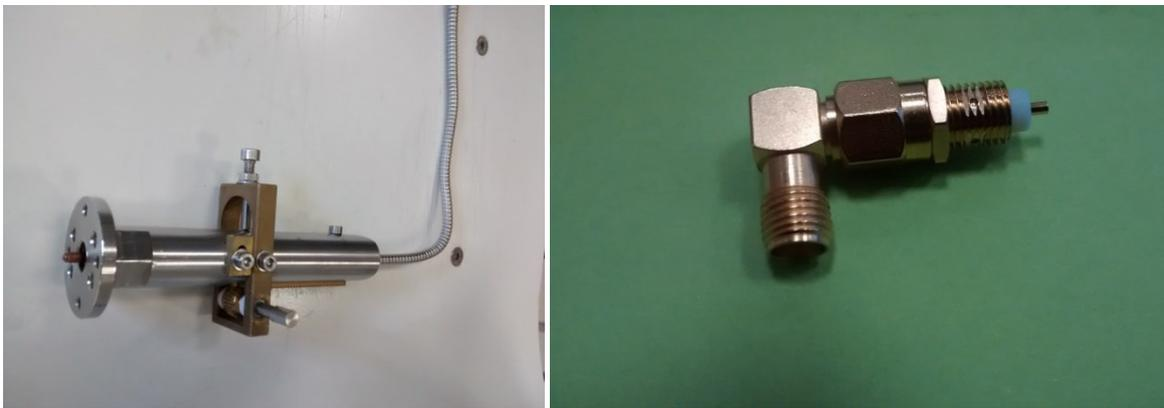
**Figure 7.6. Coupler and pick-up for the quarter wave resonator cavity.**
