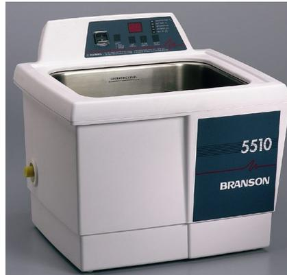
Figure 6.3 Ultra sonic bath used to clean quartz samples.
