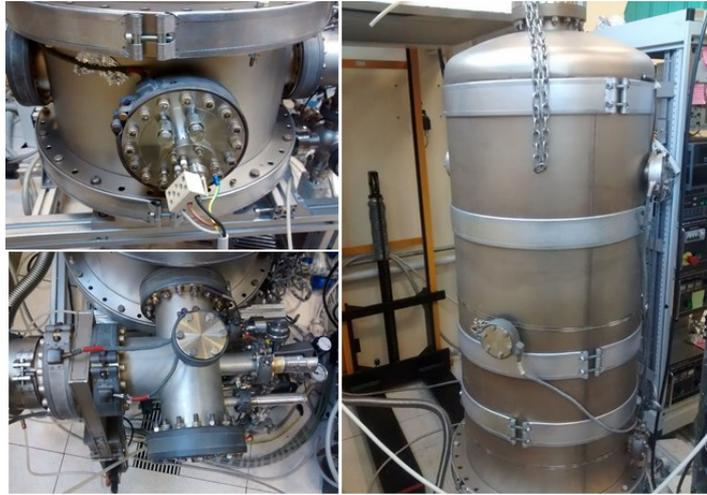
**Figure 6.8. Resistors and thermocouples placed on the vacuum chamber.**
