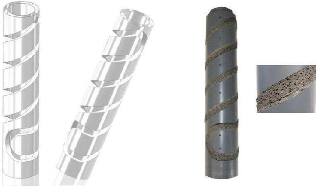
**Figure 5.6. 3D drawing of the first configuration of magnetic field. B) Neodymium- Iron –Boron placed along the double spiral path.**
