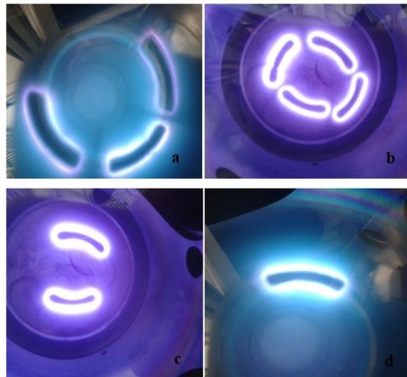
**Figure 8.6. Argon plasma produced by different top magnetic confinement. Configurations differ in the amount of magnetic material used.**
