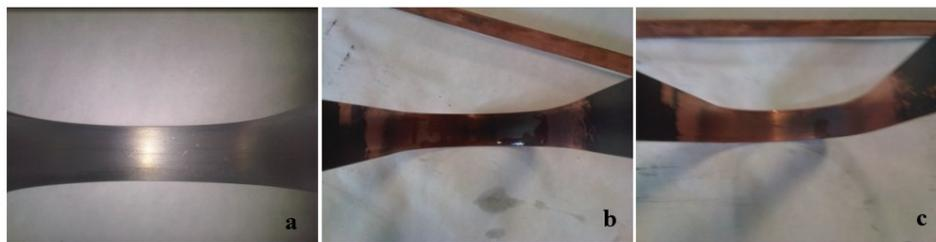
**Figure 8.2 Copper strips deposited in RUN 1. a) Before and b, c) After stripping test.**
