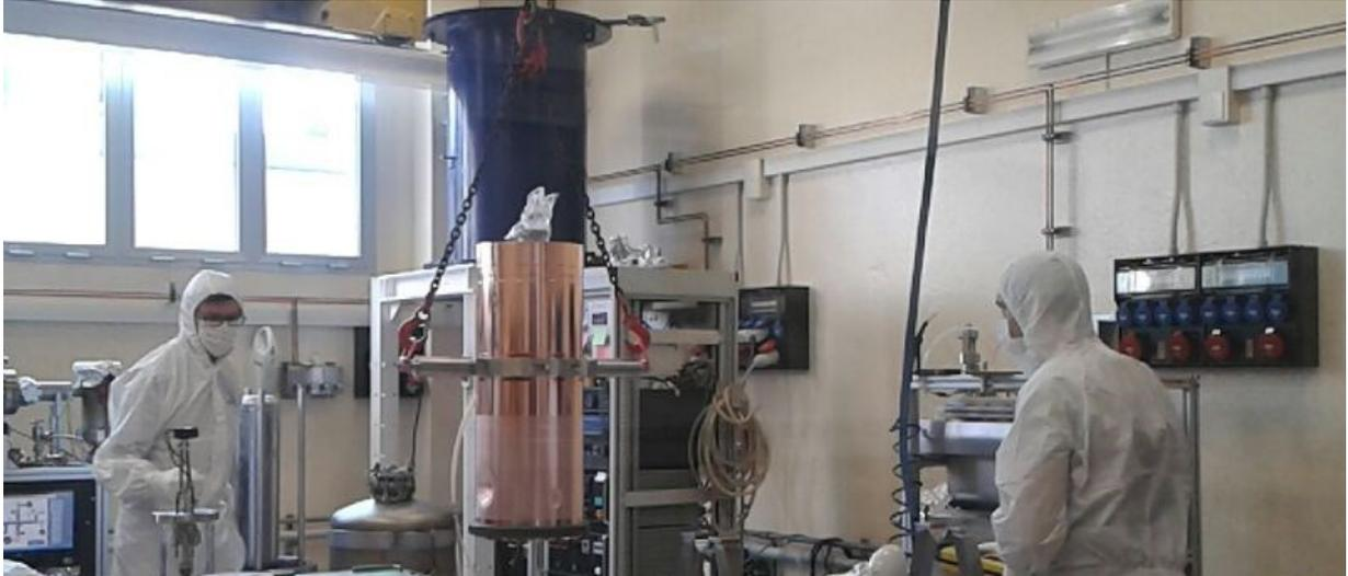
**Figure 6.15. QWR cavity during the mounting on the vacuum chamber.**
