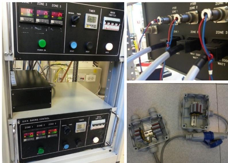
Figure 6.7. Baking controller.
