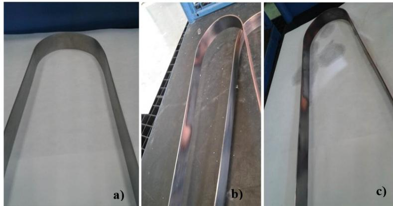
**Figure 8.11. Copper strips deposited in RUN 3, a) before and b, c) after stripping test.**
