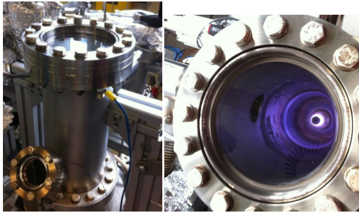
FIGURE 3.7 - PHOTO OF THE SYSTEM USED FOR TESTING THE NIOBIUM SPUTTERING PARAMETERS.
