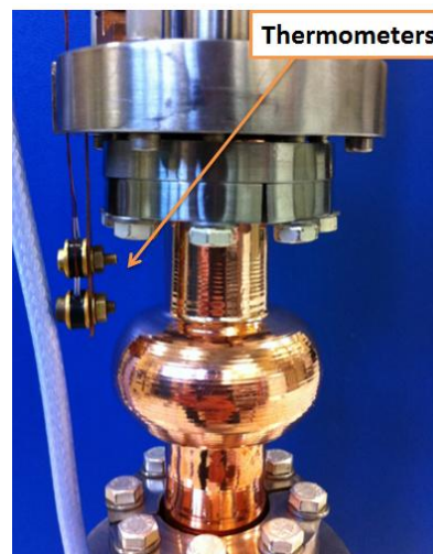
FIGURE 5.25 - CU1_2 RF TEST THERMOMETER POSITION.
