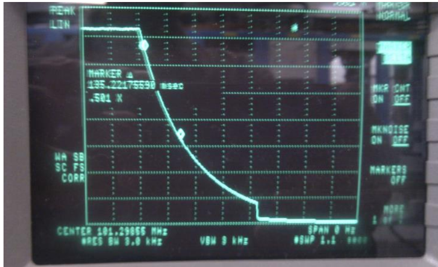
FIGURE 4.5 - VOLTAGE DECAY SIGNAL SEEN BY THE SPECTRUM ANALYZER [24].
