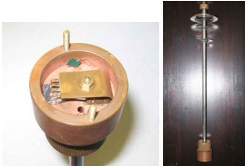
FIGURE 3.9 - PHOTOS OF THE HOLD SAMPLE AND THE PROBE FOR THE RRR AND T_c MEASUREMENTS.
