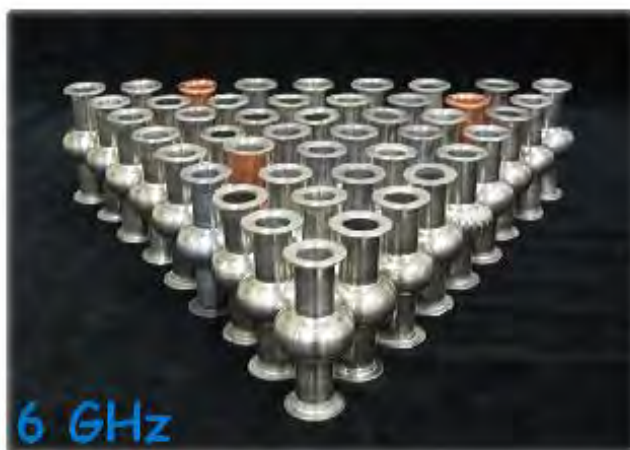
Figure 1.1. 6 GHz cavities for the RF tests 2 Surface treatments of 6 GHz cavities
