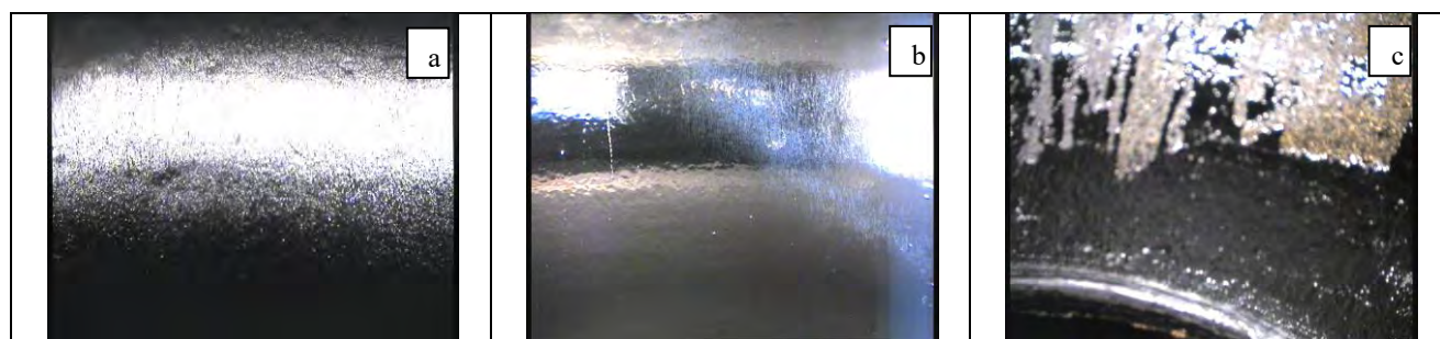
Figure 5.3. Photos after Electrochemical polishing in vertical open system (Electropolished separately): a, b – cut-off; c – cell.
