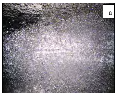
Figure 5.16. The Cell after electropolishing in the system of horizontal electropolishing whole cavity half immersed half in the solution.
