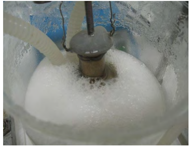
Figure 5.5. Open system for the vertical Electropolishing cavity with supply electrolyte from one side.
