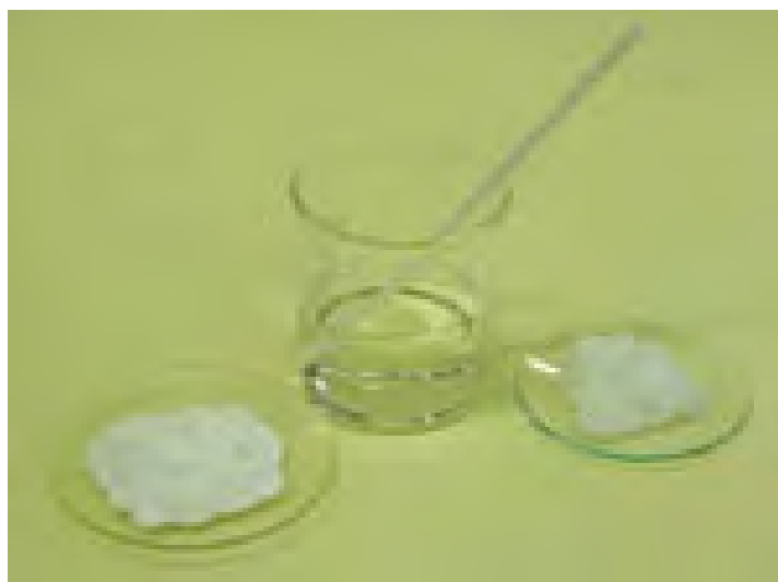
Figure 3.1. Ionic liquid that have used in this work: from the left – Choline Chloride; from the right – Urea; in the center combination both components were heated to about 100°C.
