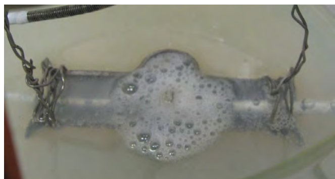
Figure 5.17. System for the electropolishing the half cavity.
