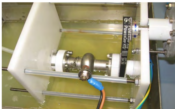
Figure 5.19. The new system for the electropolishing half of cavity.
