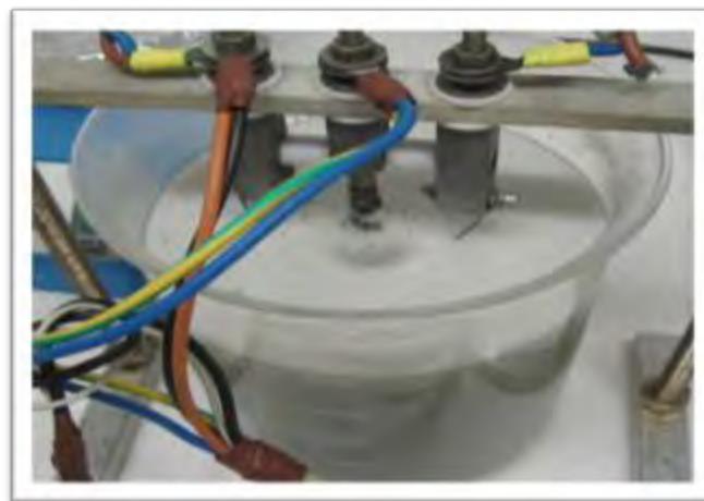
Figure 5.1. Open system for the vertical Electropolishing cavity.
