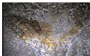
Figure 5.2. Cell after vertical Electropolishing in open system
