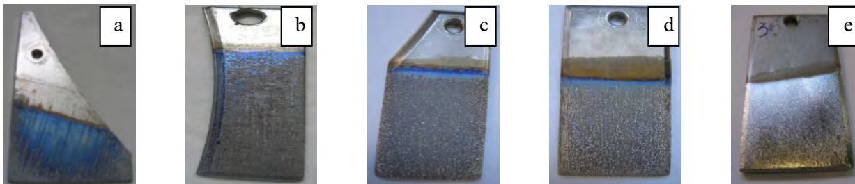
Figure 4.2. Samples Choline Chloride and Urea with small amount different additives. a – 1 ChChl : 2 Urea + 1% Tiron; b – 1 ChChl : 2 Urea + 1% Ammonium Acetate; c - 1 ChChl : 2 Urea+5 g/l EDTA; d – 1 ChChl : 2 Urea+30 g/l EDTA; e – 1 ChChl : 4 Urea + 1-2 g/l Acetylthiourea.
