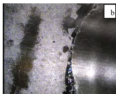
Figure 5.16. The Cell after electropolishing in the system of horizontal electropolishing whole cavity half immersed half in the solution.
