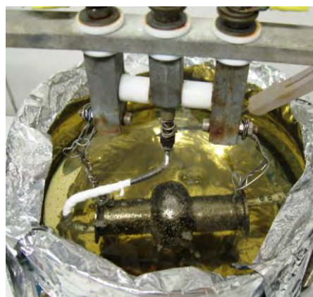
Figure 5.8. Open system for the horizontal electropolishing.
